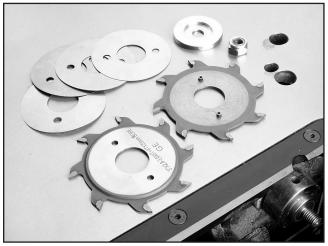
Figure 33. Scoring blade with shims.
